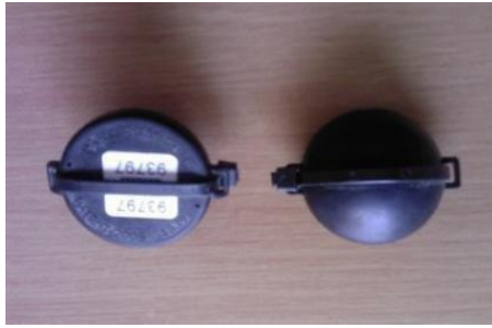
Figure 1. PARC RGM Solid State Nuclear Track Detector [10].
